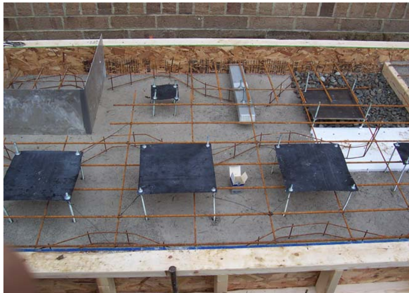
Figure 3: Test slab with purpose built defects
